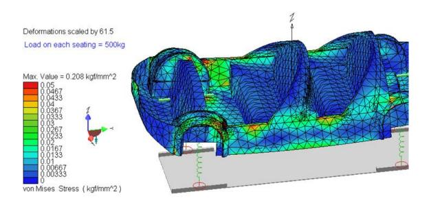
Test program: Bending 2g, Torsion2g, Shok in front1g& 10g, Shock in back1g &10g, Shock in side 2g&10g, Shock in roof 5g. Material special 3D composite sandwich.
